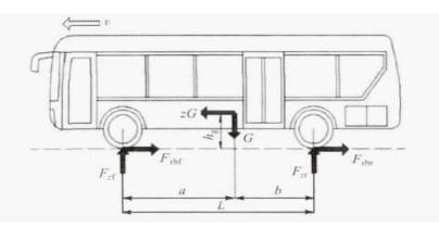
Figure 1 electric bus brake force analysis
